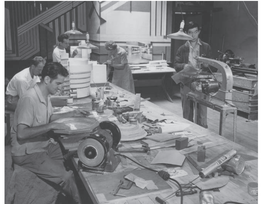
An important phase of Taliesin training was the making of models of buildings designed by Wright, like the one built in 1945 of the Solomon R. Guggenheim Museum. In a separate room off their drafting studio, Taliesin apprentices use plastics, plywood, and other materials to construct scale models of their projects. At work here are (left to right): Burton Goodrich, John de Koven Hill, Douglas Lockwood, Beatrice Reik, and Lee Kawahara.
